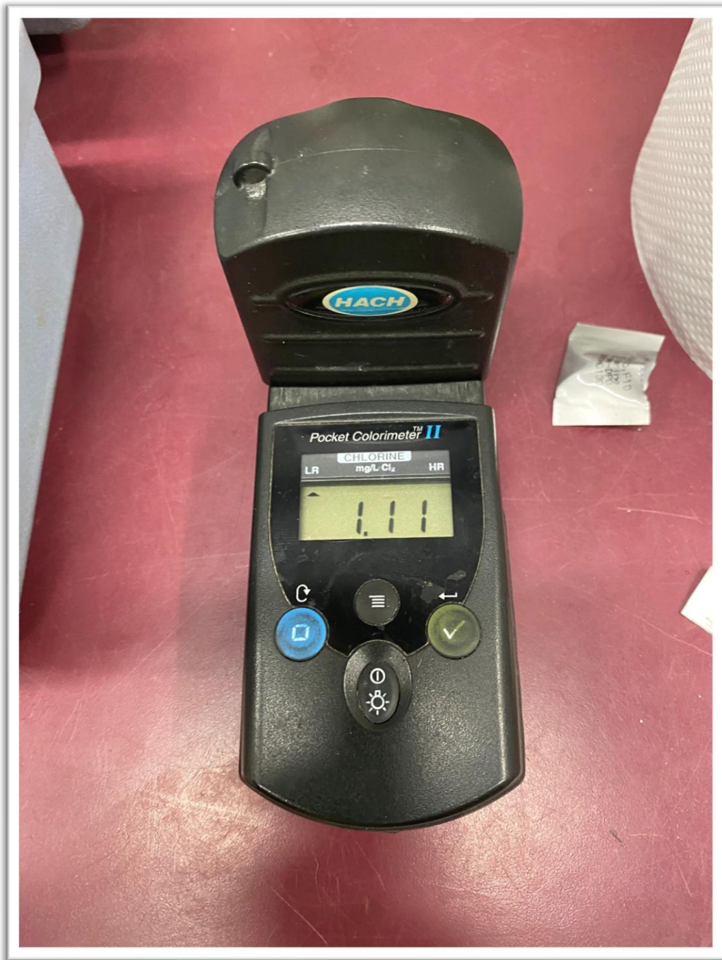
Figure 19: Verifying Reservoir Inline Chlorine Value
