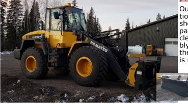
Our new loader has a multi position snow blade attachment that should make it easier to clear parking lots and other snow clean-up jobs. The blade assembly was mated to the loader in the third week of November and is ready to use in future storms.
