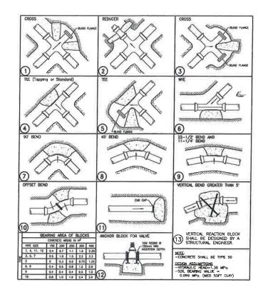
3 TYPICAL THRUST BLOCK ARRANGEMENT NOT TO SCALE
